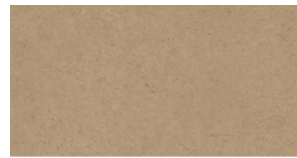
CONCRETE ochre LRV 26.8% NCS S 4020-Y10R
